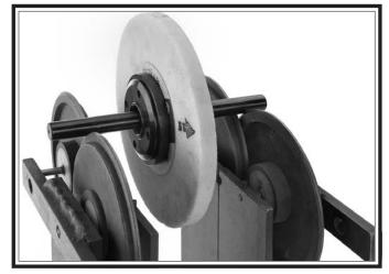
Figure 33. Wheel on balancing fixture.
